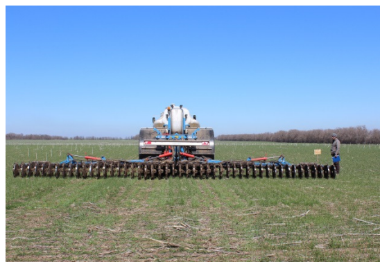
Fig. 4. Liquid nitrogen fertilizers introduction by means of Duport liquiliser
