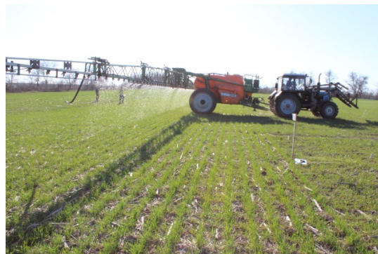
Fig. 2. Liquid nitrogen fertilizers introduction by means of trailed sprayer AMAZONE UX 4200 Super
