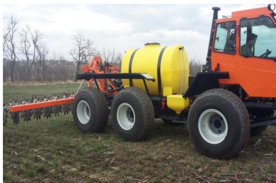
Fig. 3. Liquid nitrogen fertilizers introduction by means of multi-injector Tuman-2
