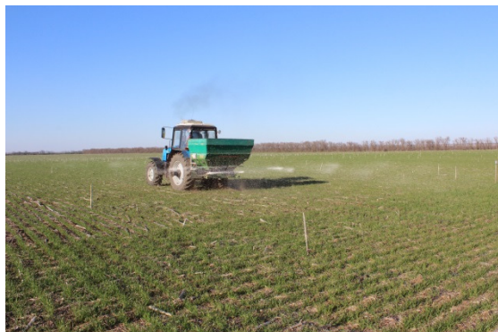
Fig. 1. Ammonium nitrate introduction by means of mineral fertilizer spreader AMAZONE ZF-M 1500
